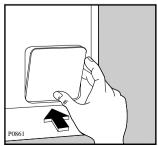
If the filter is blocked and the machine is unable to drain you will need to drain the water manually from the machine at this stage. To do this, unhook the drain hose from the standpipe or sink and hold the end of the hose over a bowl on the floor. The water should drain by gravity into the bowl. When the bowl is full, hook the hose back up and empty the bowl. Repeat the procedure until water stops flowing out.
